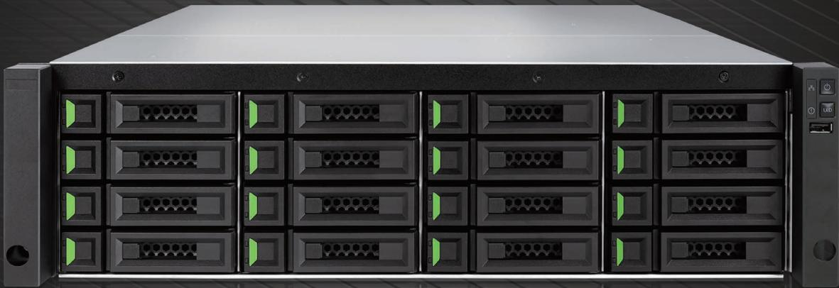
QSAN XCubeDAS XD5300 Series is a cost-effective DAS (Direct Attached Storage) or JBOD (Just a Bunch Of Disks) for server expansion. It is also a RAID expansion enclosure for QSAN SAN (Storage Area Network) XCubeSAN series.
