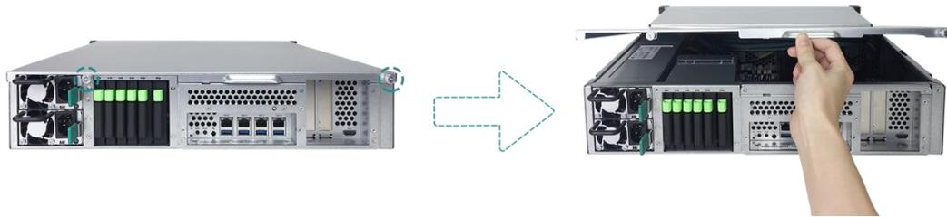
3. Remove the cable on the cable holder and remove the fan module.
